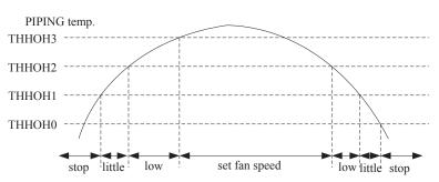
If other conditions are satisfied, when the compressor stops, the indoor system will operate at a little speed. The indoor fan will stop when the coil temperature is below the THHOT0.
