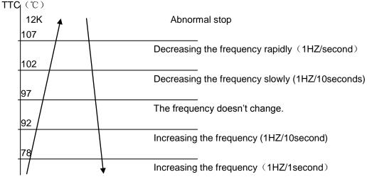
TTC>= $107^{\circ}$ C lasts for 20 seconds. Overheating protection of air-blowing, alarm malfunction to the indoor, others don't last.
