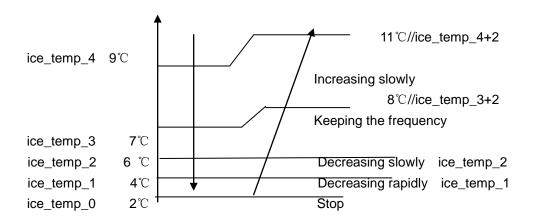
When Tpg\_indoor 〈 ice\_temp\_1, the frequency of the compressor decreases at the speed of 1HZ/1second.
