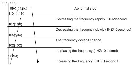
TTC>=110 $^{\circ}$  lasts for 20 seconds. Overheating protection of air-blowing, alarm malfunction to the indoor, others don't last.
